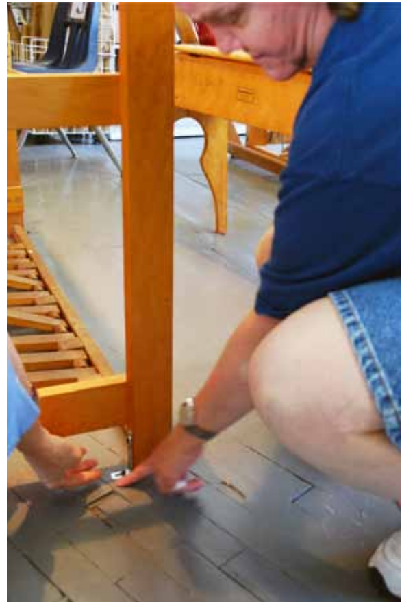
Ona points out the brackets which hold her loom fast to the floor, so that it will not move while she works.
