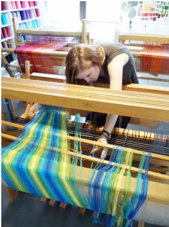
Mallory dresses the loom by threading each thread in order through wire heddles.
