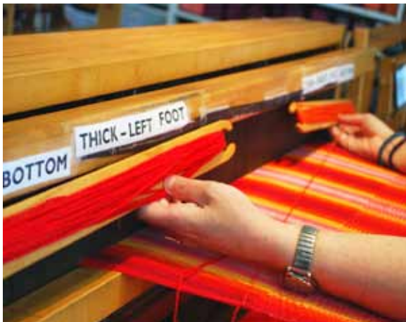
These guides act as a reminder to Ona of what her pattern is. The thick weft yarn goes through the warp from the left and the thin weft yarn goes through the warp from the right.
